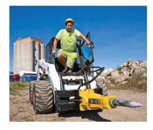
The SBU hydraulic breakers represent a unique concept in breaker technology with a patented, one-piece housing construction, the Solid Body concept. SBU breakers have an outstanding power to weight ratio and are quick and easy to position. One piecing housing also means fewer components and less maintenance.
